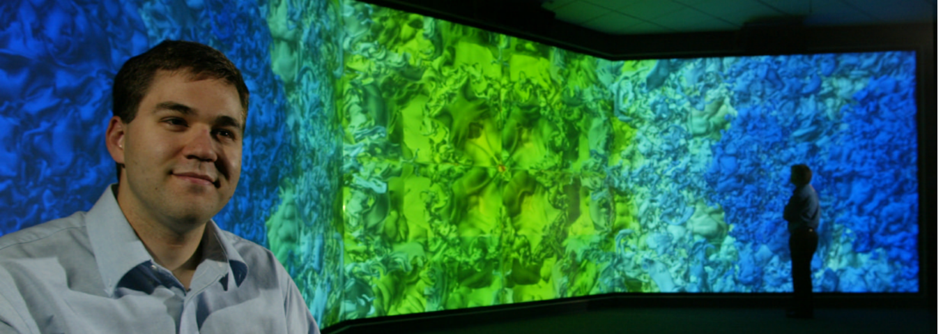
Figure 6: The VIEWS Corridor display. The display contains about 63 million pixels. The isosurface being displayed contains about 470 million triangles. Our VTK application can render this isosurface on our display in about 15 seconds. With coarser levels of both geometric and image detail, we can sustain a minimum frame rate of 5–10 Hz.
