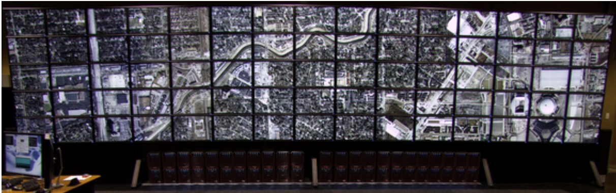
Fig. 1. Texas Advanced Computing Center's Stallion, weighing in at over 300 million pixels, is currently the world's largest display. Image courtesy of Greg Abram, Texas Advanced Computing Center.
